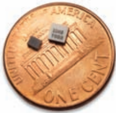
Avago Technologies' tiny RFICs have helped lead to smaller wireless products with increased battery life.
